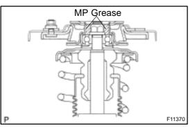
(f) Using a screwdriver to hold the suspension support, install a new nut.
